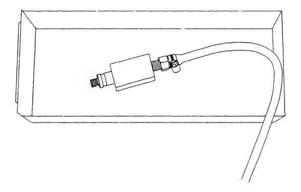
If no fault is found, re-install constant pressure valve in pump.
